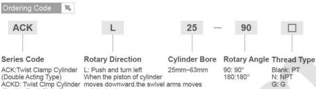
ACK:Twist Clamp Cylinder (Double Acting Type)
